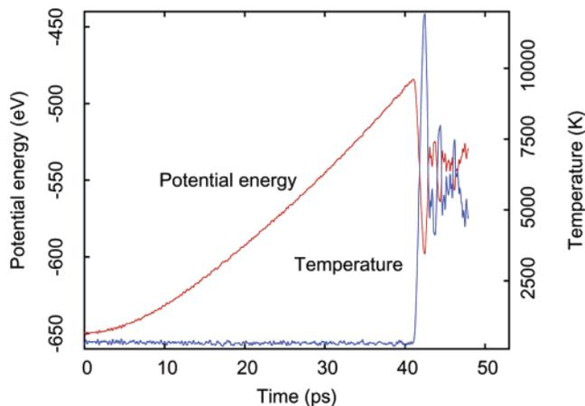
**Figure 4.** Potential energy and temperature versus time for the MD simulation of the stretching of a perfect (4,4) tube.
