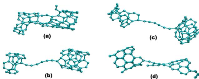
**Figure 3.** Several structures obtained by stretching a (4,0) nanotube with a Stone–Wales defect (left) or a vacancy (right).
