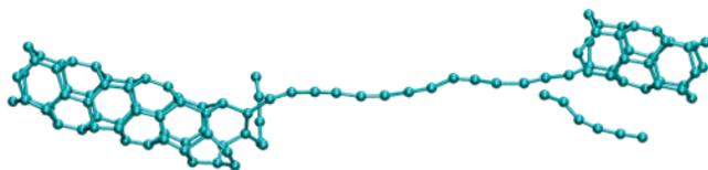
**Figure 5.** Figure of a fourteen atom wire formed by stretching a (4,0) tube containing two vacancies. One can also observe a six atom chain that detached from the tube.
