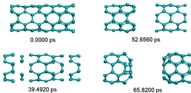
**Figure 2.** Simulation at 1500 K of the breaking of a (4,4) tube. The sequence shows the nanotube in the equilibrium geometry, breaking of the tube, and capping by fullerene-like structures. Note that “bonds” between atoms are drawn if atoms are closer than 1.7 Å and should not be interpreted as real chemical bonds.
